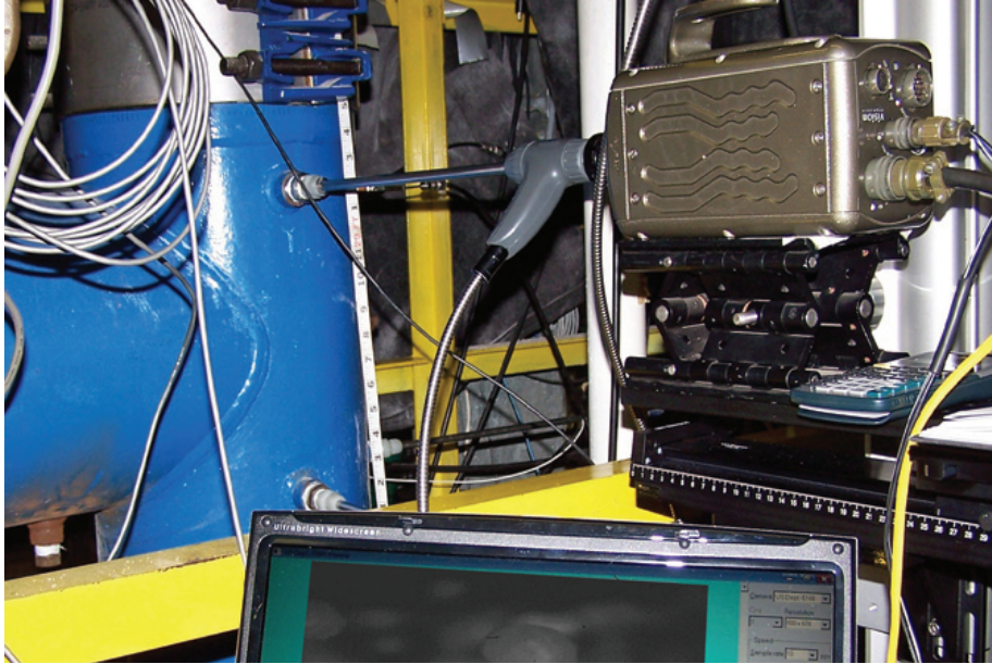
Phantom v7.1 high-speed camera applied to a cold flow gasification experiment at the NETL.
